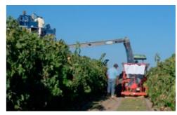
**4. PAPER TRAY LAYER** The tray layer hopper spreads the grapes evenly, one or two grapes thick, onto a continuous paper tray for even and faster drying. The continuous paper tray typically runs the entire length of the row, usually a quarter mile or longer (approximately 430 meters).
