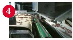
LASER SORTER Laser sorters remove stems and other foreign materials with precision accuracy.
