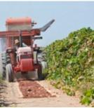
When the grapes have dried into raisins, a machine picks up the raisins from the continuous tray, transfers the raisins into bins in the next row, and shreds the paper tray so it can be incorporated into the soil.
