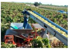
3. OVER THE ROW CONVEYOR When the grapes are shaken from the vine by the machine harvester, they are conveyed over the vine row to the tray layer and placed in the tray layer hopper.
