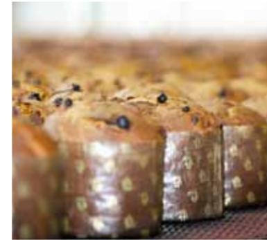
4. The dough rises again after being placed in paper molds, and is then transported into the oven by conveyor belts.
